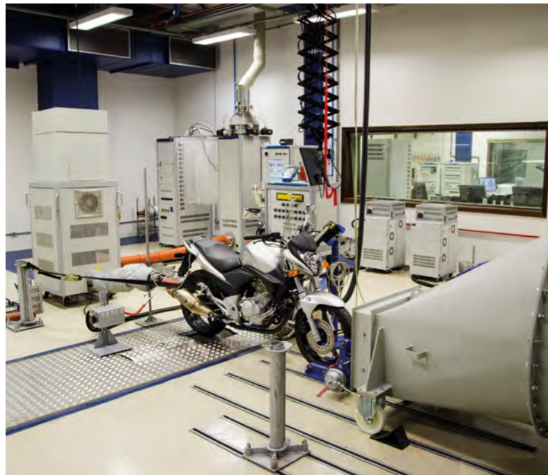
Test of emissions of a motorcycle realized at one of the Lactec laboratories © Lactec
