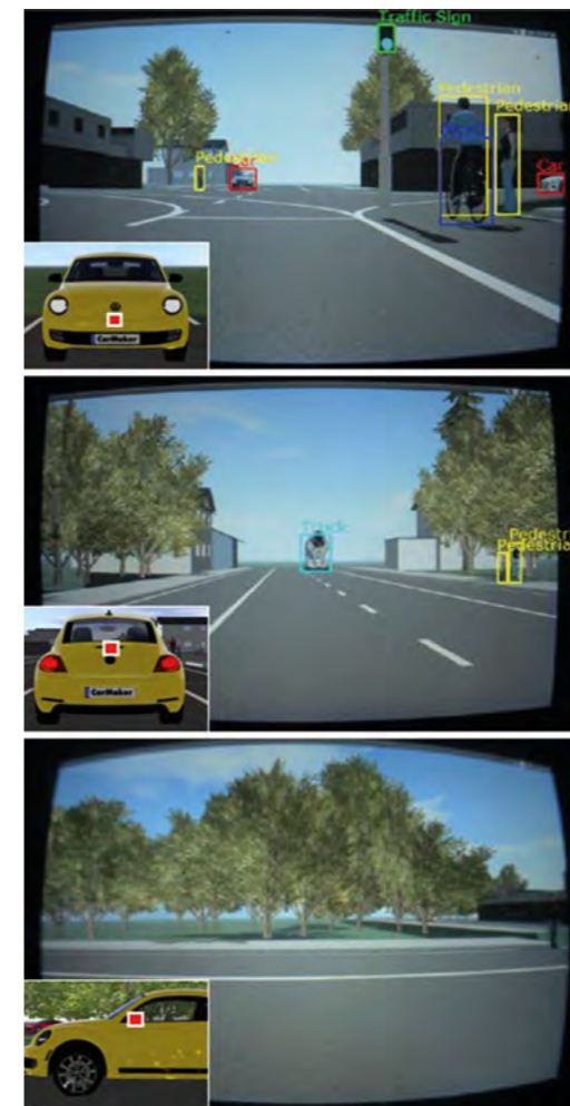
Simulation-based testing of an ADAS algorithm for detection of traffic participants © Fabio Reway
